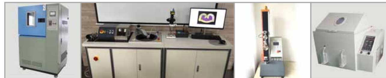
IP等级测试仪 protection degree tester 剖面分析仪 Metallographic analyzer 拉拔力测试仪 Pull out force tester 盐雾腐蚀试验箱 Salt mist tester
